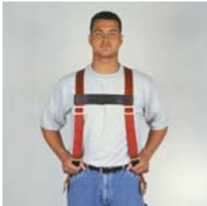
Figure 5 - Attach chest strap to keep shoulder straps parallel and held in position so the harness cannot slip off in a fall.
