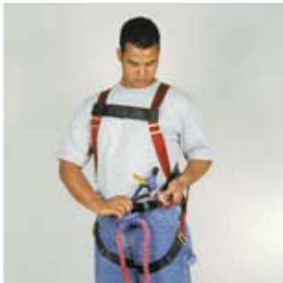
Figure 8 - Attach the carabiner through the fabric web loop at the end of the shock absorber or connecting lanyard. Then attach the Rope Grab Knot to the carabiner through the black plastic Rope Thimble. BE SURE THE CARABINER IS LOCKED.
