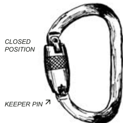
FIG 2 GATE AND LOCKING SLEEVE IN CLOSED POSITION
