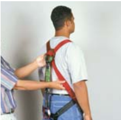
Figure 7 - The area on the harness where the Nylon Ring or D-Ring is attached is called the Chafe Pad. It should be located just below your shoulders in the center of your upper back area as shown in the photo above. Adjust as needed for proper fit.
