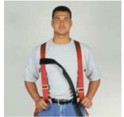
Figure 3 - With shoulder strap buckles facing forward, put on the harness as you would a jacket. The D-Ring or Nylon Ring should be properly located on your back. Adjustments are easier if you get help when first setting up the equipment.
